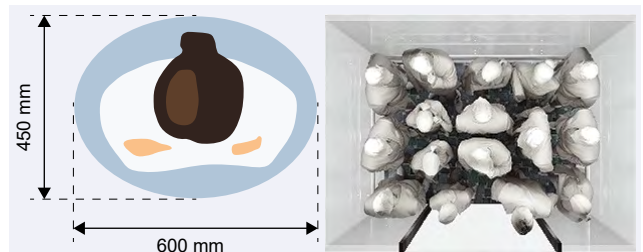
Figure 3 The space occupied by each person in a fully loaded lift car Courtesy of: (left) D2E and (right) Hoare Lea
